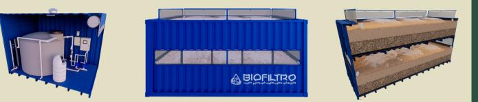
We design and provide Control Units, which include an equalization tank, pH adjustment system, solid separator, pump station, PLC, and sensors, to feed our two story twenty foot long "Wiggle Room" treatment modules. Each Wiggle Room houses worms, microbes, wood shavings, and an irrigation system while the two floors can act in parallel or series to accommodate seasonal volume and strict discharge requirements.
